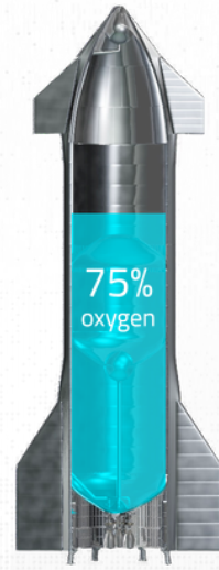
SpaceX's Starship rocket and the percent mass made up of oxygen (Courtesy Helios )
